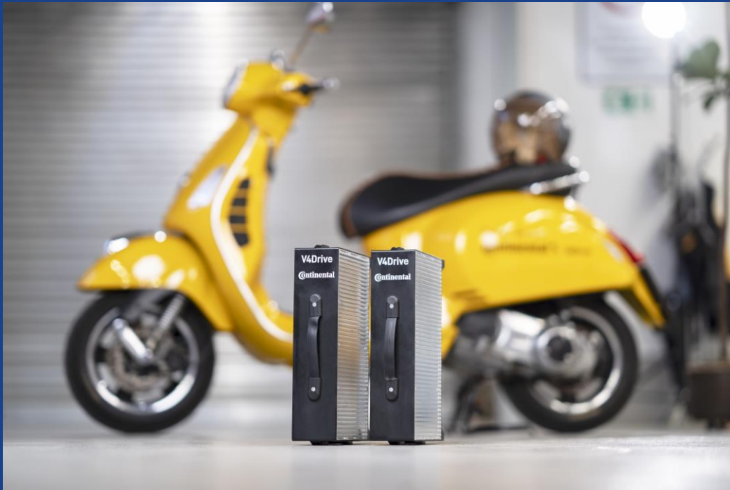
New 48-volt battery pack in front of an electrified scooter. Copyright: Continental
